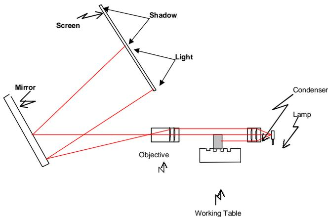
Students should view the operation of an optical comparator to observe how it is used as a quality tool.
