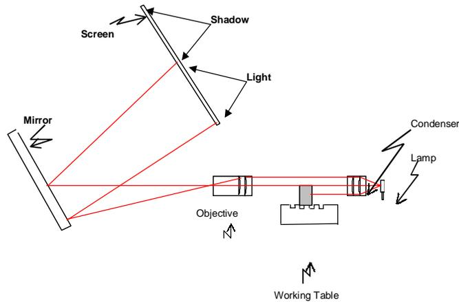
The part to be inspected is placed on the working table, and a concentrated, parallel beam of light intercepts it. The light beam then passes through the objective lens and is refracted so that it will focus on the screen. The front surface mirror serves only to reflect the beam so that the screen can be placed in a convenient location for viewing.
